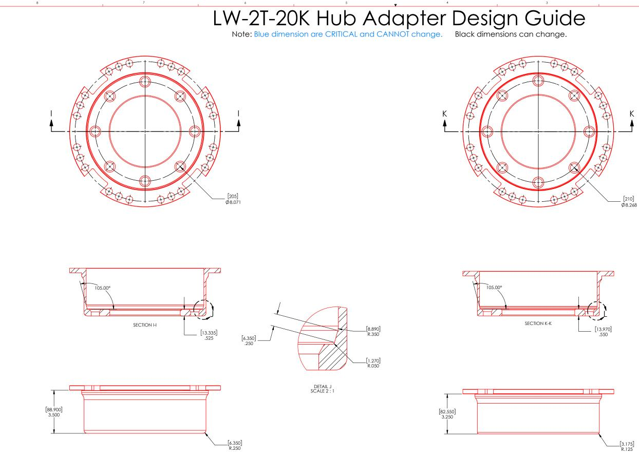
It is essential that the adapters match the recommended guidelines. This will ensure the system can withstand the rated loads and provide the most accurate results. The critical features are shown in blue. Customers may change all other geometry. Examples of permitted changes are shown above.
