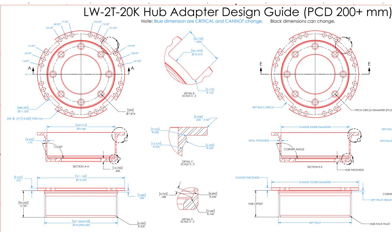
It is essential that the adapters match the recommended guidelines. This will ensure the system can withstand the rated loads and provide the most accurate results. The critical features are shown in blue. Customers may change all other geometry. Examples of permitted changes are shown on the second sheet. This design guide is for vehicles with a PCD greater than or equal to 200 mm.
